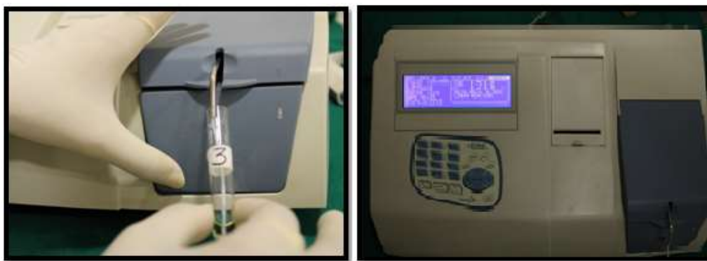
Figure 3: Prepared solution analyzed in semi automatic biochemical analyzer machine (Erba Mannheim Chem 5x)
